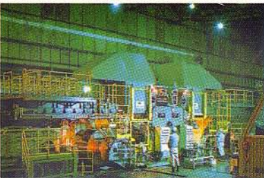
Three sets of 20-high Sendzimir cold rolling mill - to meet diverse range of rolling requirements.
