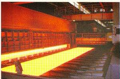
Two thick plate annealing furnaces conduct heat treatment under optimum conditions for products of every type and size, and supplying top-quality products.
